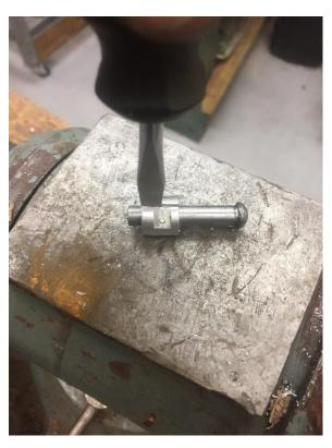
When done machining the part, I released it from the collet by forcing the flat blade screwdriver into the side slot.
