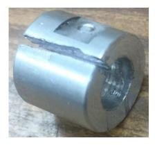
To make the collet, I mounted the scrap aluminum in my 3 jaw chuck and drilled it through using the closest size drill. It didn't matter if it was a little over or under.
